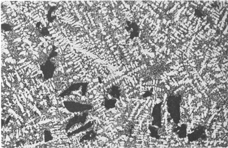
Figure 5 Graphite particles are distributed in the interdendritic regions. Matrix alloy Al-7.2% Si-2.2% Cu with 2% graphite. (90 X).
